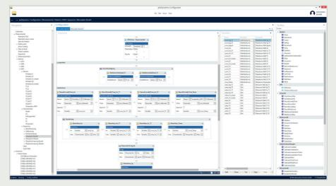
The configurator allows an intuitive configuring and parameterizing of the hardware incl. online-status. In addition, test plans, measure- and calibration- sequences could be created and changed with a graphical editor without programming knowledge. An extensive function- library (toolbox with drag- and drop- function) helps to create complex measuring- sequences. A text- editor can apply customized algorithm.
