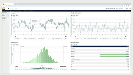
The web-visualization including extensive analytics- and statistical functions (quality control chart, measurement statistic, detailed results, measuring curve etc.) is intended for monitoring the product quality. Warnings and events are displayed in plain text with a record history. An online hardware-status and a real time display of sensor values makes troubleshooting easier. Parameter-changes are applied according to user authorization and would be logged.
